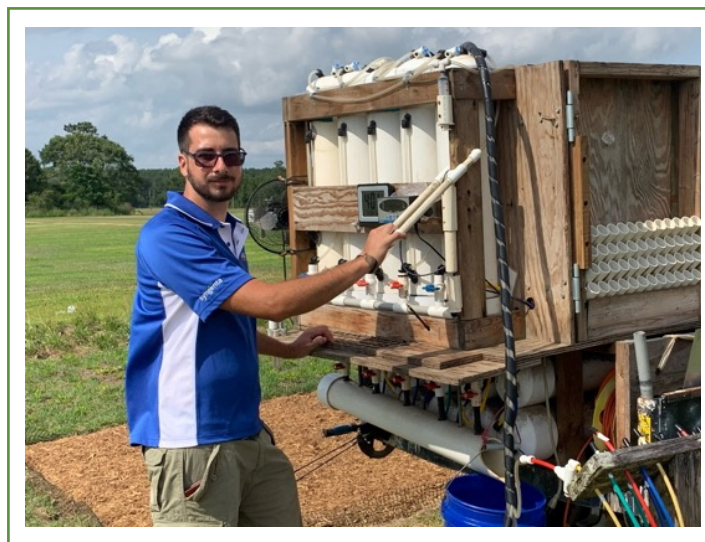
Figure 2. Pumping station utilized to collect water leachate samples.
