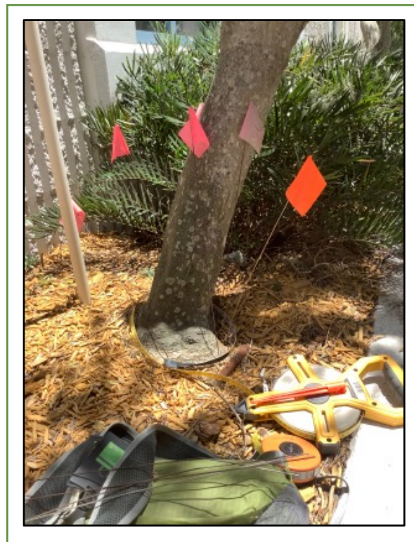
Figure 1. Image of the field method for measuring the circumference of the trunk flare.
